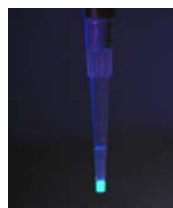
Fluorescently labeled IgG captured on the affinity resin of a PhyTip 200+ column
