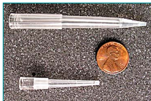
Figure 3. PhyNexus PhyTip columns, 200+ and 1,000+ sizes
